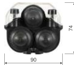
Dimension of connection box type TB-1 and TB-2 [mm]
