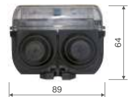
Dimension of connection box type TB-11 and TB-12 [mm]
