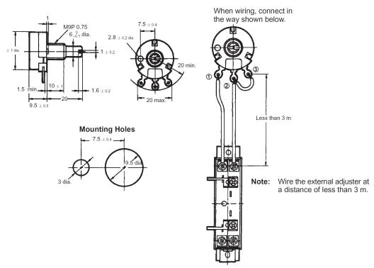
Note: When using the external adjuster for input, be sure to set the input selection slide switches accordingly.
