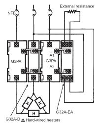
3. Control Using Internal Adjuster
